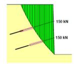
$\rightarrow$  Use a factor of  $(\frac{1}{2})$  to distribute the 3-D Loading for a 2-D analysis
